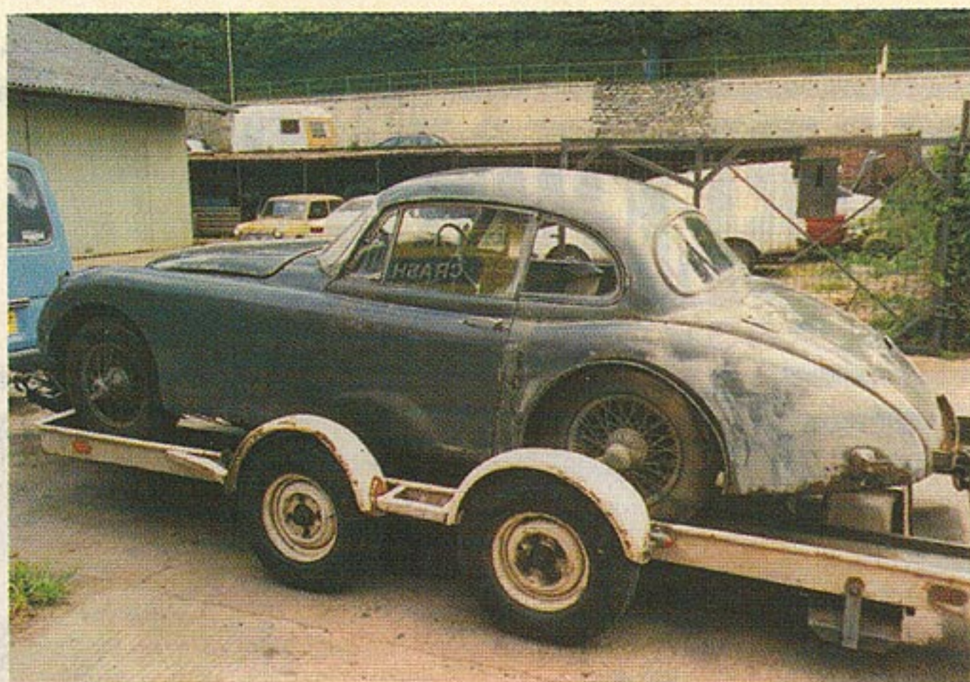
1958 Jaguar XK150 remained complete, but body corrosion was extensive
