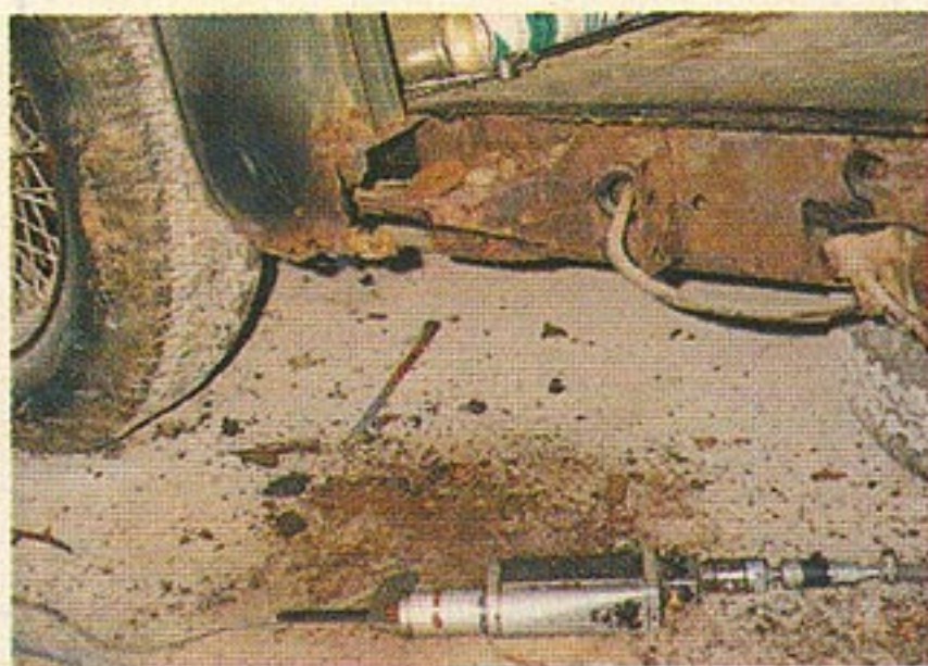
1958 Jaguar XK150 remained complete, but body corrosion was extensive
